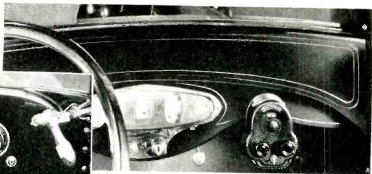
(Above) In this type of receiver the controls are encased in a neat metal box easily attached to the instrument panel.
